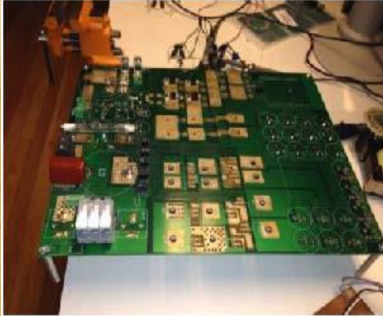
Product #2—DC to AC 98% Efficient Smart Inverter
