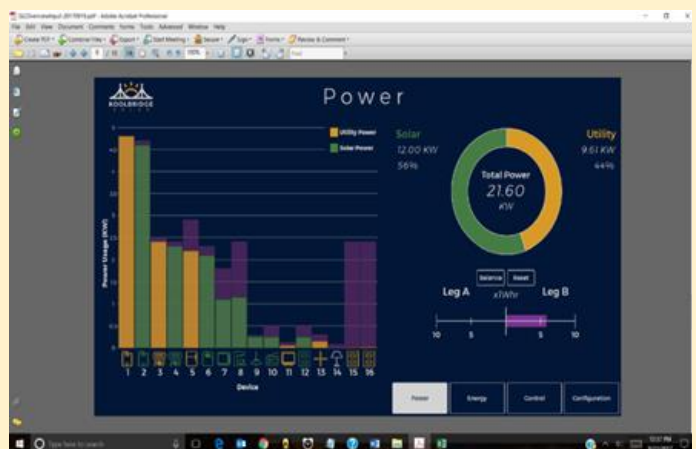
Figure 4. Laptop screen display showing power consumption monitored by the SMART LOAD CENTER
