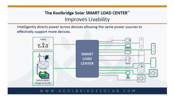
In the future, it is anticipated that more and more Smart Appliances will emerge and Koolbridge Solar is preparing to be able to communicate between the microcontroller in the SMART LOAD CENTER and such Smart Appliances to control when or how they will operate. High power-consuming appliances would be logically controlled to operate when there is free solar energy available as opposed to expensive utility power.
