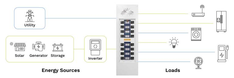
Typical installation showing SMART LOAD CENTER's Patented Dual Bus Architecture, sharing Utility to some loads and alternate energy to different loads simultaneously.
